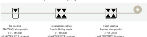
GEBECON™ felting needles used for pre-needling offer the perfect combination of good surface properties in the end product and optimum bending strength. Treating the felting needles with GEBEDUR™ II over the complete needling process guarantees an extended service life and consequently a uniform needling effect for the whole application period.
