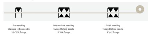
The twisted working part of a Twisted felting needle ensures greater barb definition in application. The result: more efficient intermediate and finish needling and consequently capacity for higher production speeds.
