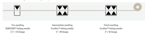
GEBECON<sup>TM</sup> felting needles used for pre-needling offer the perfect combination of good surface properties in the end product and optimum bending strength. The use of EcoStar<sup>TM</sup> felting needles for intermediate and finish needling results in the best possible surface quality.
